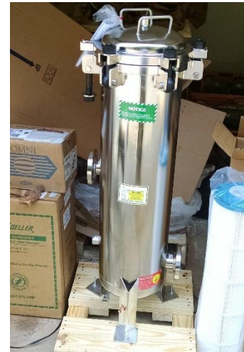
New cartridge filter for upgraded filtration plant.
